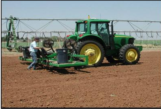
Figure 9. Installation of SDI laterals with GPS guided tractor, TAES, Halfway, 2006.
