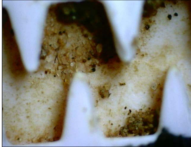
Figure 3. Deposits of sand particles with no indications of MnO 2 precipitation in a magnified drip emitter pathway, TAES, Halfway (picture taken in 2005).
